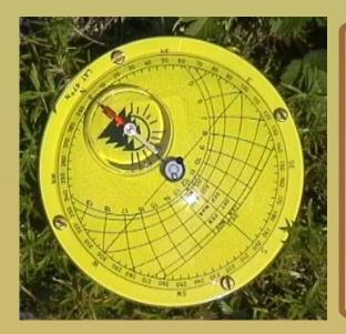
The sun compass is made of a yellow anodized aluminium slice of 116 mm diameter with a black printed scale.
